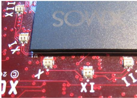
**Figure 4.4:** Closeup of the LEDs
