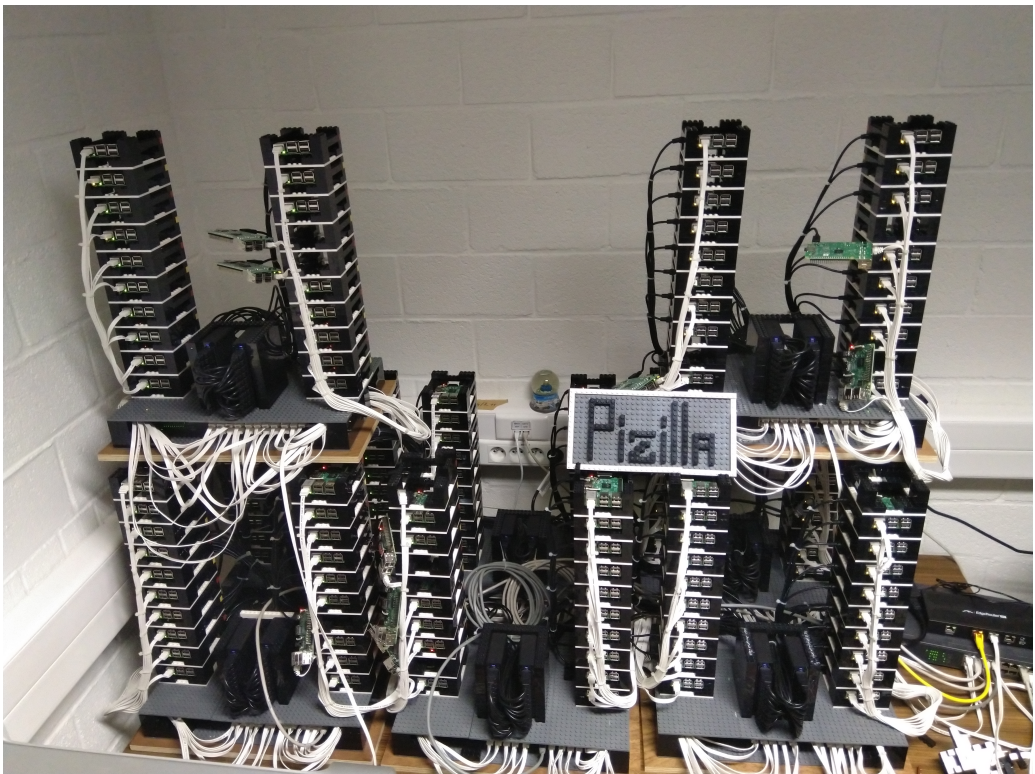
Figure 6.11.: Photo of the Raspberry Pi cluster. The Raspberry Pis are encased in LEGO®.
