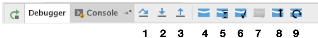
Figure 5.13: Stepping commands. Sequential stepping: (1) step over (2) step into (3) step out. Message stepping: (4) step to message receiver (5) step to promise resolver (6) step to promise resolution (7) step next turn (8) return from turn to promise resolution (9) step end turn.
