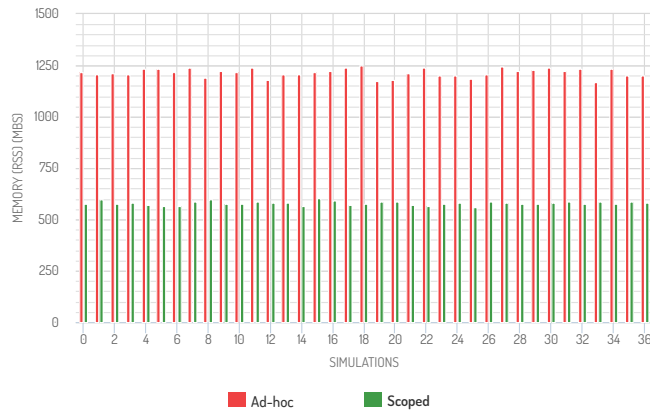
(c) Memory (resident set size) consumed by both approaches over all simulation runs.
