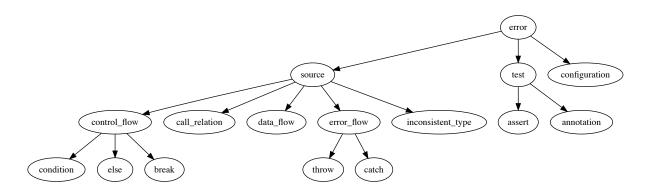
Figure 1: Example of a category hierarchy of code integration errors.
