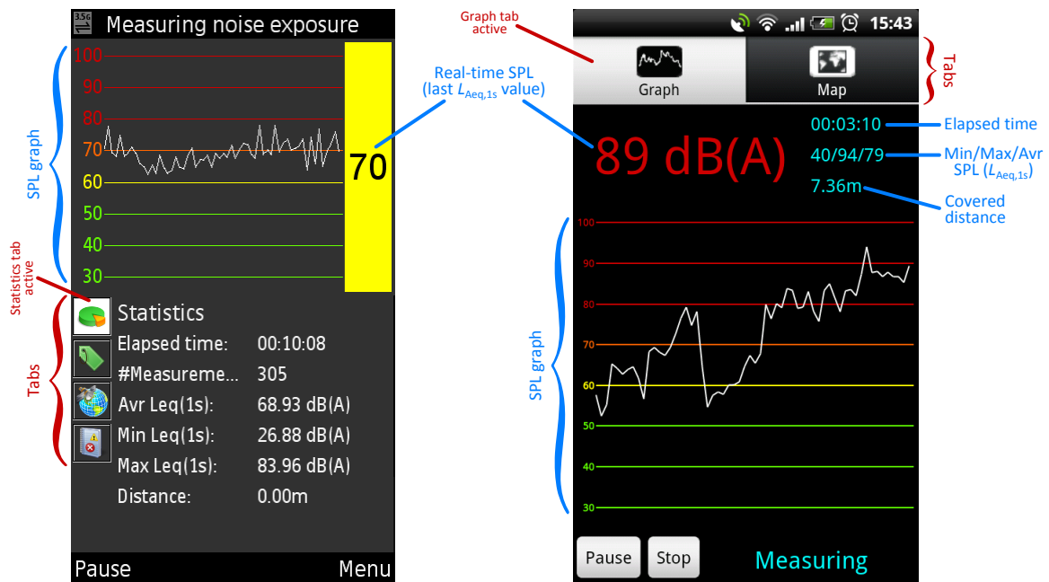
Figure 6.2: Measuring sound pressure level with NoiseTube Mobile (Java ME variant on the left, Android variant on the right)
