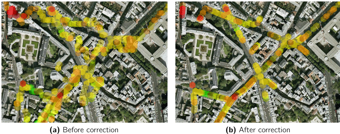
Figure 5.2: Correction of GPS coordinates through map matching
