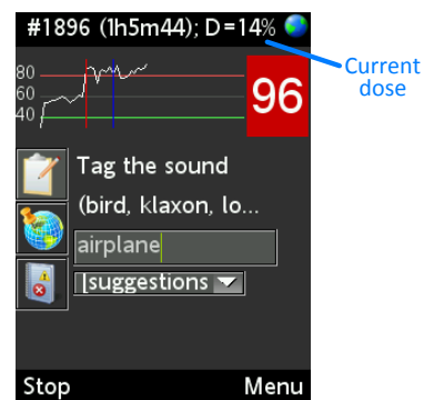
Figure 6.8: Experimental dosimeter feature in Java ME app
