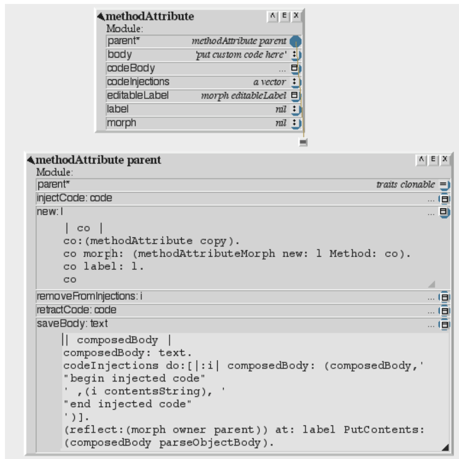
Figure 6.3: The methodAttribute prototype and its parent.
