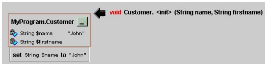
Figure 2: This figure shows the a newly created customer object using the standard visualization. The current executing method (denoted by the arrow) is showing the constructor method ( init ). The customer's first name has been initialized.
