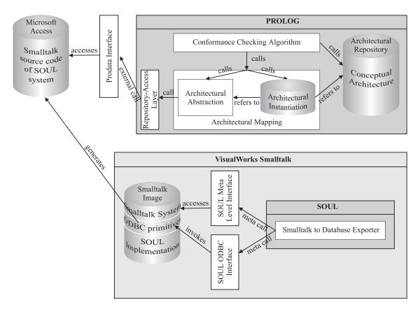
Figure 6.3: Setup for conformance checking in PROLOG.
