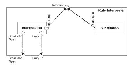
Figure 6.5: Bindings for the 'Rule Interpreter' sub-architecture.
