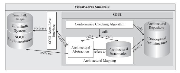
Figure 6.2: Setup for conformance checking in SOUL.
